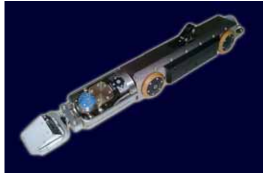
A typical Grinding Robot with onboard CCTV monitoring system. Picture courtesy of PMO, Switzerland.
