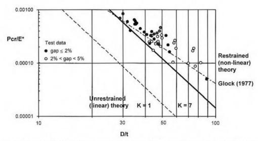
Figure 4. Aggarwal's 1984 buckling data compared contemporary theories (source Gumbel (2001))
