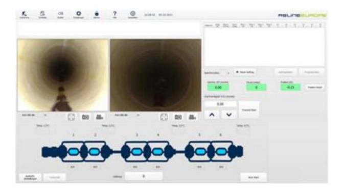
Figure 7: Real-time monitoring of the whole curing process
