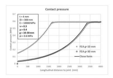
Figure 7. Contact pressure versus longitudinal distance to joint and gap.
