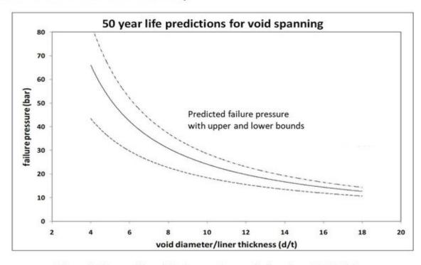
Figure 7. 50-year life void/hole spanning predictions for a PE 80 lining.
