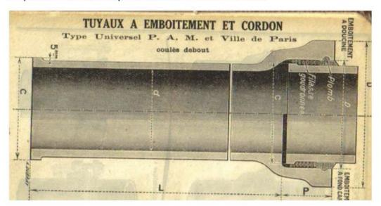
Figure 1. Gray cast iron pipe with bell and spigot and with lead caulked joint. Extract from the 1920 Pont-à-Mousson catalog.
