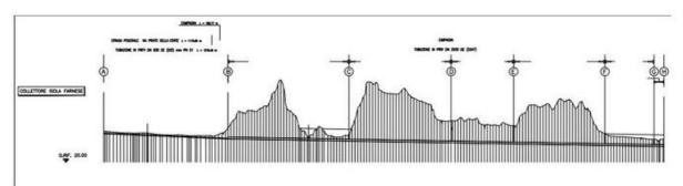
Figure 2. Profile for DN2000 pipe, showing topography and location of shafts
