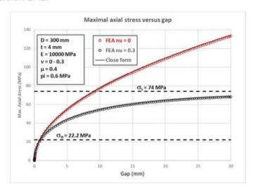
Figure 3. Maximal axial stress versus gap and Poisson's coefficient.
