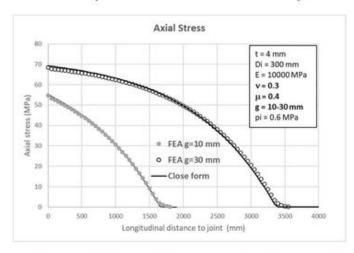
Figure 5. Axial stress versus longitudinal distance to joint and gap.
