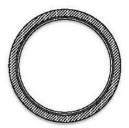
Figure 3. Liner constrained by the host pipe
