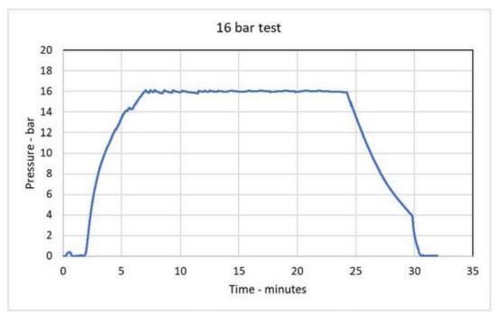
Figure 11. Fifteen minutes 16 bar test
