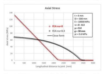
Figure 6. Axial stress versus longitudinal distance to joint and Poisson's coefficient.
