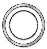
Figure 2. Liner unconstrained by the host pipe
