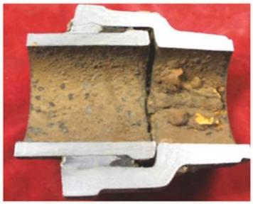
Figure 6. Gap in spigot and socket joint.
