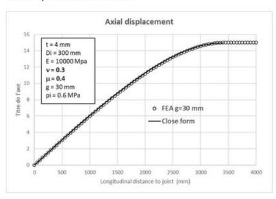
Figure 9. Axial displacement.
