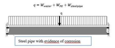
Fig.5: Steel pipe with evidence of corrosion
