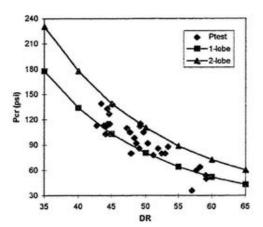
Figure 4. Comparison of predicted and observed buckling pressure from Zhao 1999.
