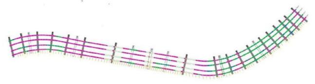
Fig.4: planimetric diagram of the pipes inside the bridge, with indication of the measured thicknesses
