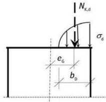
Figure 6. Parabolic stress distribution in the contact zone of longitudinal transom cracks [DWA-A 143-2].
