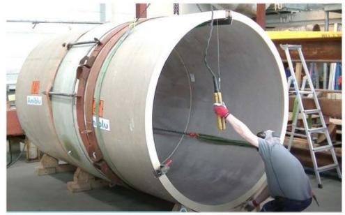
Figure 7. Assembly and adjusting angular deflection
