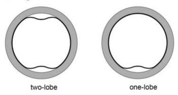
Figure 2. Typical buckling modes.
