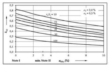
Figure 9. Diagram for determining kv,s as a function of the joint ring deformation w<sub>GR,v</sub> [DWA-A 143-2].
