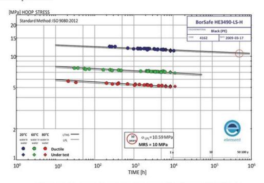
Figure 2. 50-year extrapolation in Element test report P-09/38-v2.
