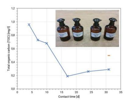
Figure 4. Data set of SAERTEX-LINER® H2O, measurement of TOC in contact water with time
