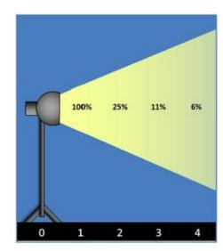
Figure 3: Drop of UV-light intensity
